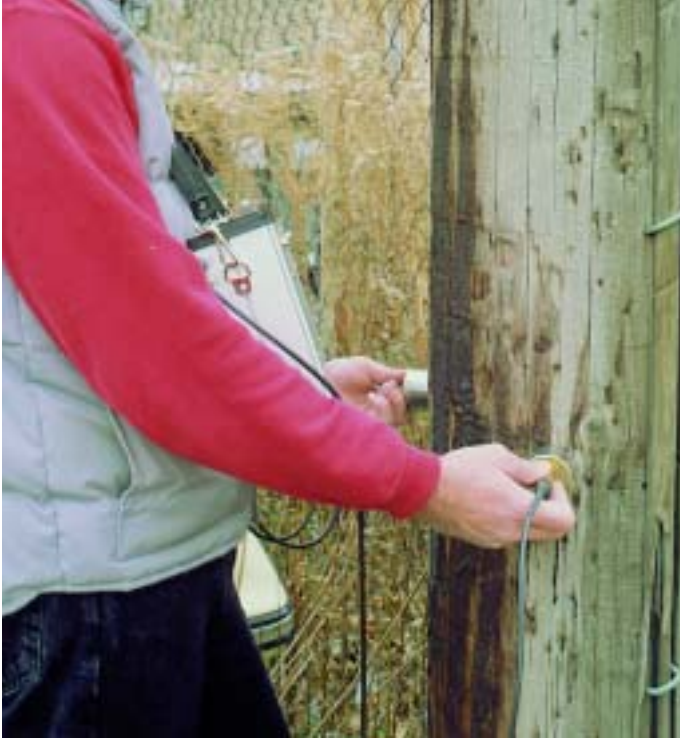
Direct method used in detecting decay and rot in wood ...
