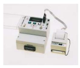
M-3056 maturity system connected to a field printer
