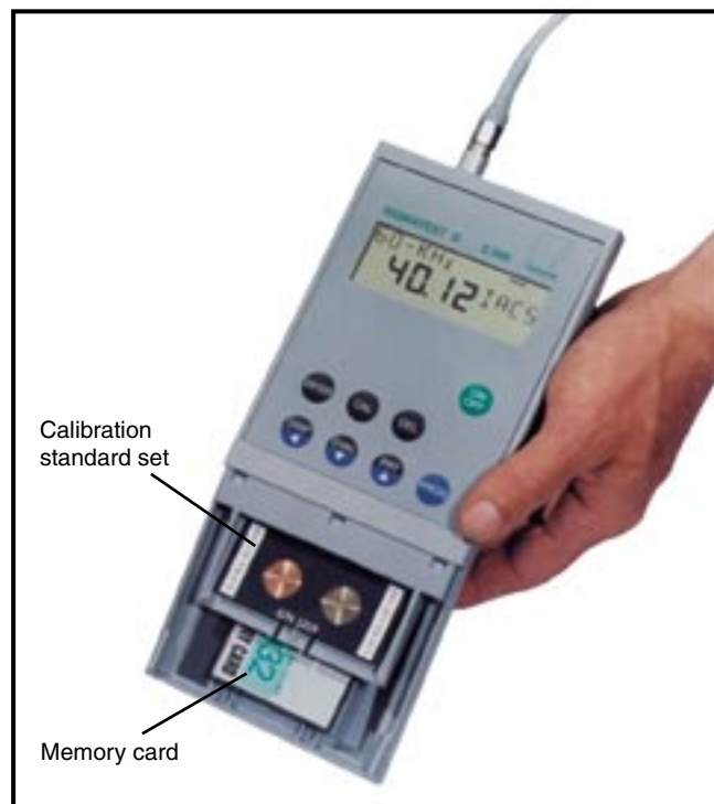
• Figure 2 - SIGMATEST D, housing opened, calibration standard set and memory card visible
