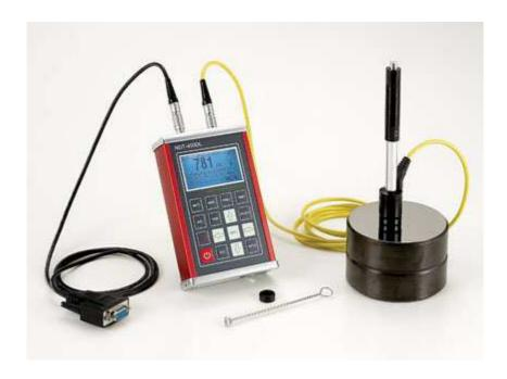
NDT-400DL is an advanced hand-held portable hardness tester, featuring: compact size, high accuracy, wide measuring range and simplicity of operation.
